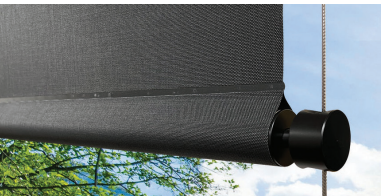
ROUND HEM BAR, Pocket (Hem Bar: 1½" diameter; pocket size: ¾")
